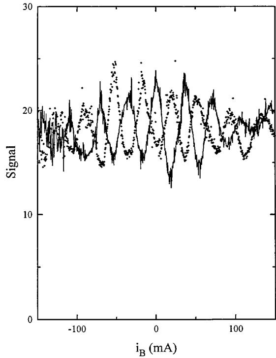
FIG. 5. Interference patterns obtained with velocity-selected atoms, by scanning the magnetic field in the phase object. Solid line, the analyzer is set at point *M* in Fig. 2(a) (central bright fringe); dots, a positive pulse is applied to TA within a time interval such that all selected atoms classically see it. The whole interference pattern is reversed.
