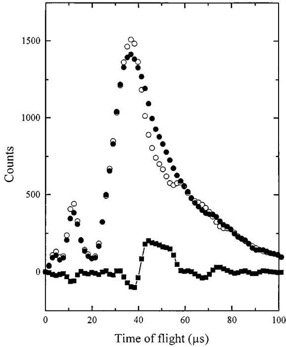
FIG. 3. Time-of-flight distributions obtained with a zero-magnetic field in the phase object. The analyzer operates under the conditions defined by point *M* in Fig. 2(a) (solid circles). When a positive pulse is applied to TA a dark fringe is obtained for all atoms that classically “see” this pulse (open circles). Solid squares denote the difference.
