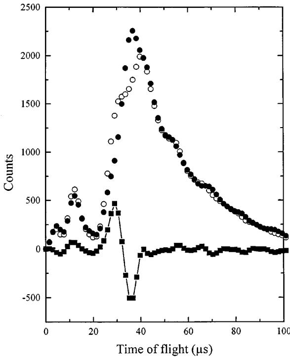
FIG. 4. Same as Fig. 3, but now the magnetic field in the phase object differs from zero ( $i_B=100$  mA). Under static conditions of analysis (open circles) interference fringes modulate the time-of-flight curve. When the TA pulse is applied (solid circles) the fringes are reversed for all atoms that classically see the pulse. Solid squares denote the difference.
