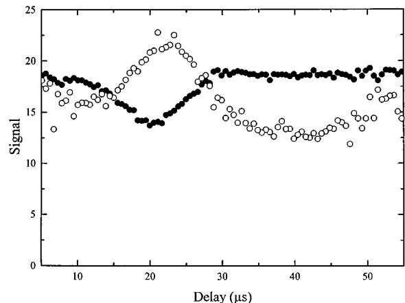
FIG. 6. Reversal of the central fringe when the delay between the starting time of the source and that of the TA pulse is scanned. Solid circles,  $i_B=0$  (dark fringe with the TA pulse present); open circles,  $i_B=56$  mA (bright fringe with the TA pulse present).
